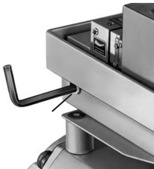
Fig. 19: Tightening feedback lever
